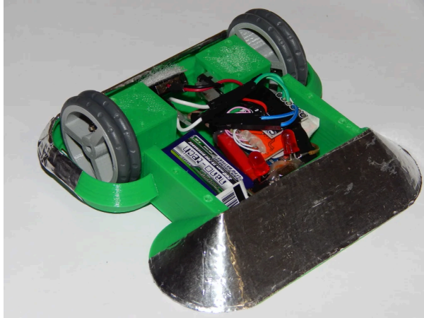
Figure 2. This robot is not eligible for participation – exposed design (battery and wires).
